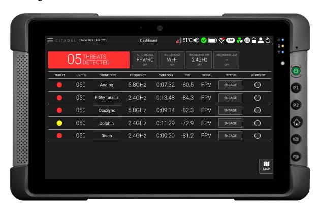
Factors that can influence RSSI values include transmitted power, receive sensitivity, physical obstacles, distance between transmitter & receiver, interference from access points in radio environment, radio interferences, and orientation of the antenna.
