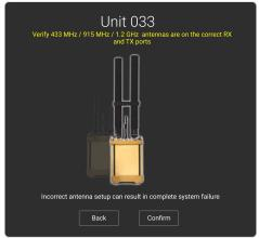
The first step is to make sure that all antennas are securely tightened to the unit following the visual diagram in the User Interface (UI). It is critical to make sure they're all tight - loose antennas will result in signal loss or unidentified / unmitigated drones. Pay close attention to the frequency selection screen (above) to ensure you have correctly connected the antennas to the RX/TX/Wi-Fi and GPS ports.
