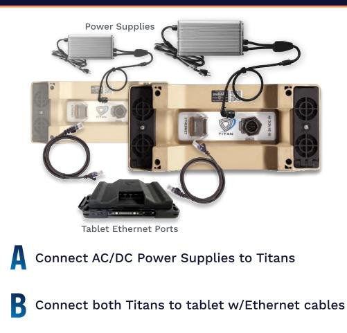
**C** Plug power supplies into AC outlets - Titans will power on automatically
