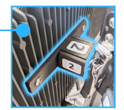
NOTE: mount devices from bottom to top for tripod stability
