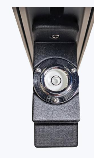
The tripod legs are independently adjustable for uneven surfaces, and the base has a bubble level to assist with alignment before loading equipment.
