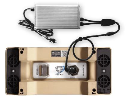
Via the same bottom panel jack, connect two 10AH 5590 batteries per system using the provided dual battery cables. (Connect the batteries to the cable before plugging into the Titan.)
