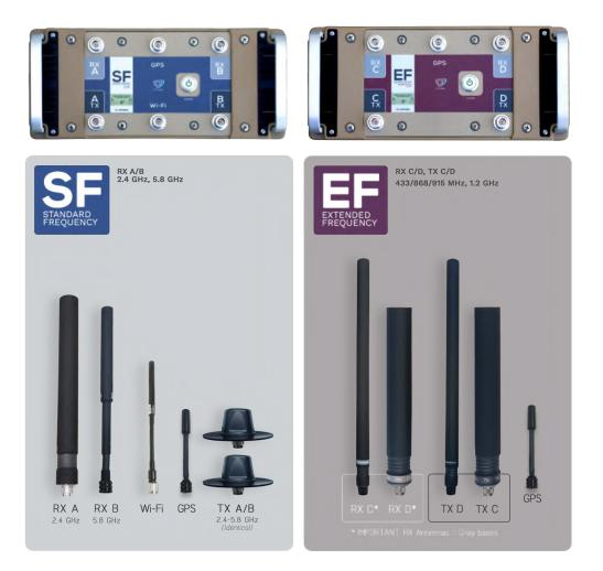
The first step is to make sure that all antennas are securely tightened to the unit following the visual diagram in the User Interface or the provided User Guide. It is critical to make sure they're all tight - loose antennas will result in signal loss or unmitigated drones. Pay close attention to the frequency selection screen to ensure you have correctly connected the antennas to the RX/TX/Wi-Fi and GPS ports.
