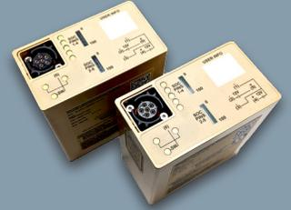
The more the system engages (transmits), the faster the batteries deplete. We've provided estimates below, but actual run time will vary with battery capacity, duty cycle, and ambient temperature. The batteries can be 'hot swapped' individually while the unit is operating to extend run time. Note that Titan does *not* recharge batteries - a separate charger is needed. Avoid running a unit on one battery unless very briefly for hot swapping.
